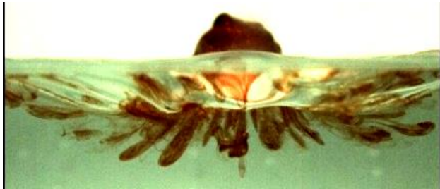
Inclined fiber loops under the primary cavity of a drop impact with chemical reaction (Doklady RAS, 2021, 66(10))
